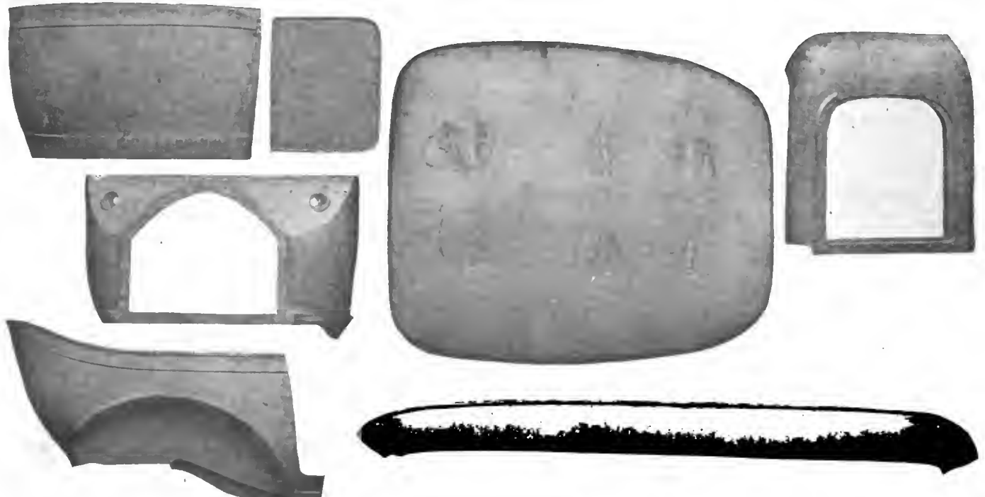
Cast aluminum parts of the new Cadillac coupé body mentioned in The Automobile for Feb. 24
